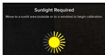
3. At this point you need to fill up the sun meter by pointing the Structure 3D Sensor outside into sunlight. If there is not enough sun light available, after five seconds you have the option to Enable Indoor Mode. Calibration only begins once you have a split screen displayed.
