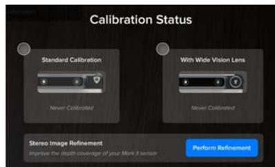
4. You will be guided through a small explanation of Stereo Image Refinement. Swipe through the tutorial and stand about one metre away from the wall and point the Structure 3D Sensor towards the wall and tap Start Refinement.
